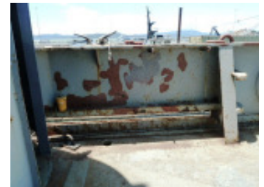
Port side gunwale before painting.
