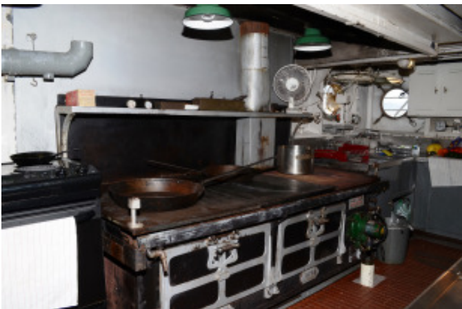
A view of the Red Oak's galley showing the original, WWII-era, Diesel-fueled stove—one of very few left in the country. . Still operational ... living history. Photo by Dori Luzbetak.
