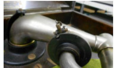
*Close-up of the taper tube with sound box and needle in up-ended, rest position.*
