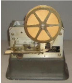
Main Gallery. The topic is fire alarms. The item not on display is a critical part of the early fire alarm system in Richmond; it is a 1928-type, triangle punch fire alarm register made by the Gamewell Co.
