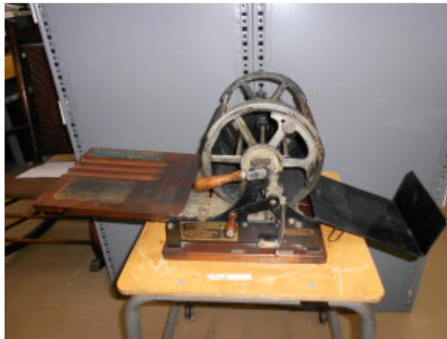
The rounded-top case measures 16 inches long, 13 inches wide and 14 inches high, plus handle. Basic operating instructions are glued to the wooden paper-feed tray and more detailed instructions are glued inside the case. Four latches secure the case to the wooden base making the unit portable.
